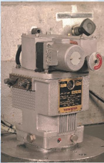
The main role of the governor is not to increase or decrease the speed which can be done via fuel control system but once the speed of the engine has been set, the job of the governor is to maintain that speed despite the variations in load.
